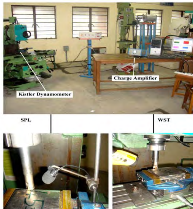
Fig.1. Hard milling process experimental setup
