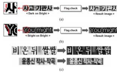
Fig.8. Process of inverting image by the color polarity. (a) Dark text on bright background. (b) Bright text on bright background. (c) Examples of inverted text by “bright_text_flag”.
