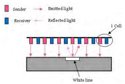
Fig. 2: Working principle of line following algorithm
