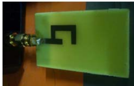
Figure 6: Fabricated printed G-shaped monopole antenna
