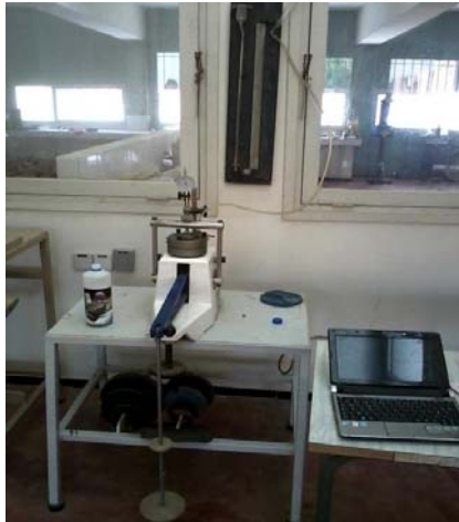
Fig. 4. Oedometer apparatus and equipments used in the test
