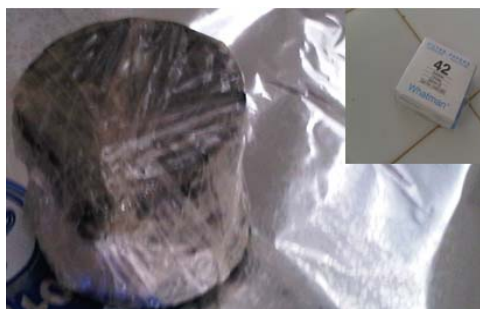
Fig. 5. The system “filter paper-soil” carefully protected will be in bag to avoid the influence of rays
