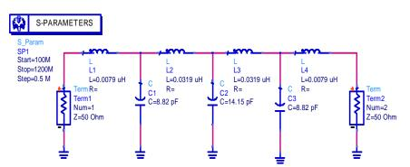
Fig 3. Butterworth low pass filter before tuning cutoff at 450MHz
