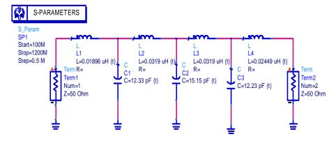
Fig 4. Butterworth low pass filter after tuning cutoff at 450MHz
