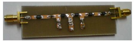
Fig 10. Hardware Butterworth low pass filter
