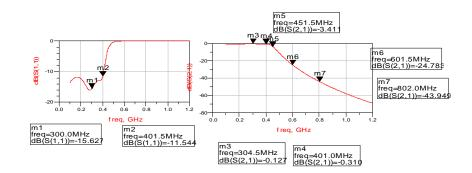
Fig 5. Actual simulation S-parameter result before tuning
