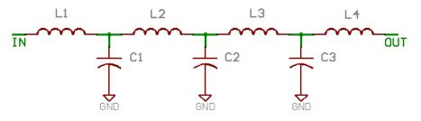
Fig 2. The 7 poles circuit design by filter calculator
