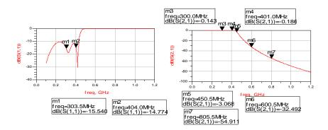
Fig 6. Simulation S-parameter result after tuning
