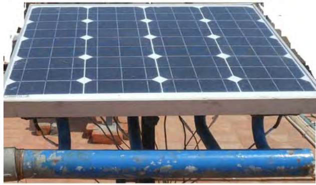
Fig 3. Photographic view of the PV panel with cooling channels and headers
