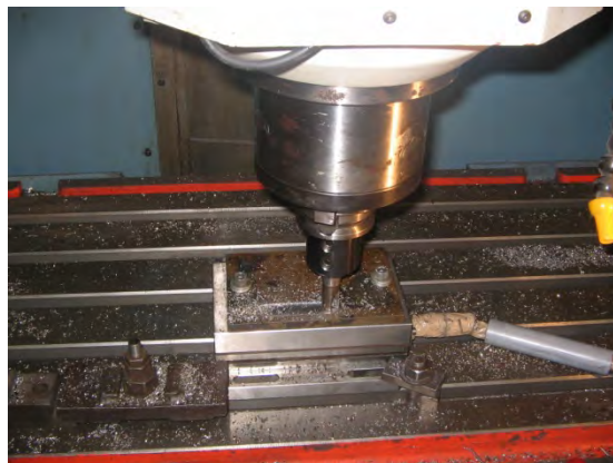
Fig. 3 Work piece mounted on Dynamometer
