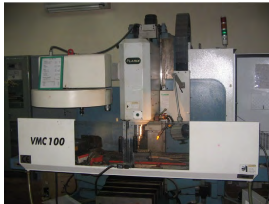
Fig. 1. ARIX VMC100, 3 Axis Vertical Machining Centre
