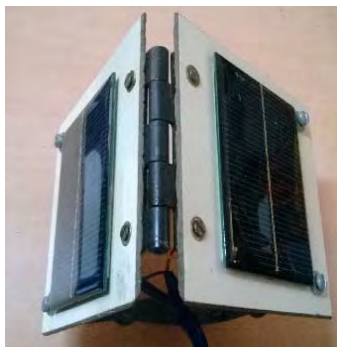
Fig. 2 Arrangement of PV cells for tracking
