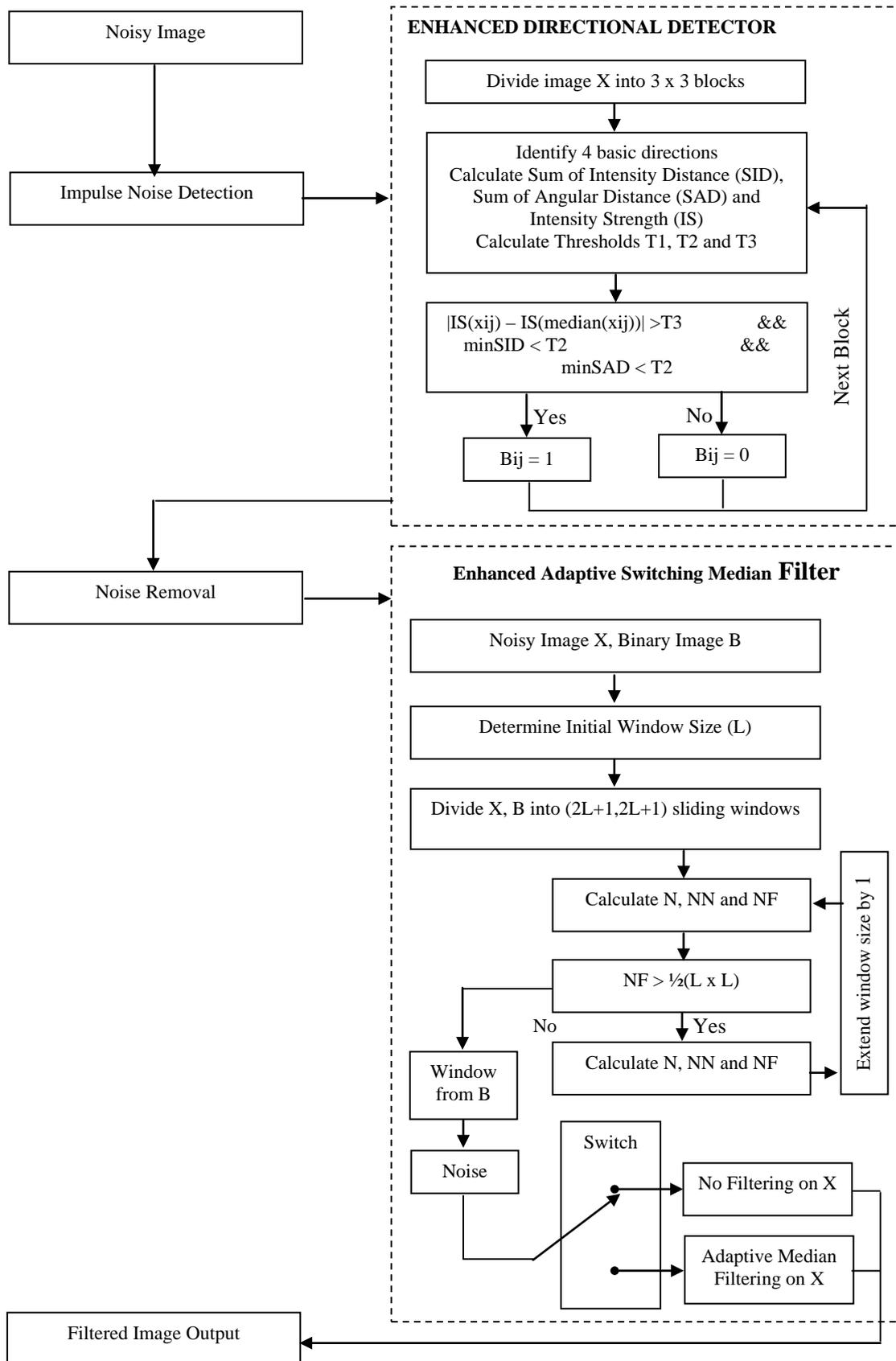
Fig 2. Enhanced Directional Switching Median Filter
