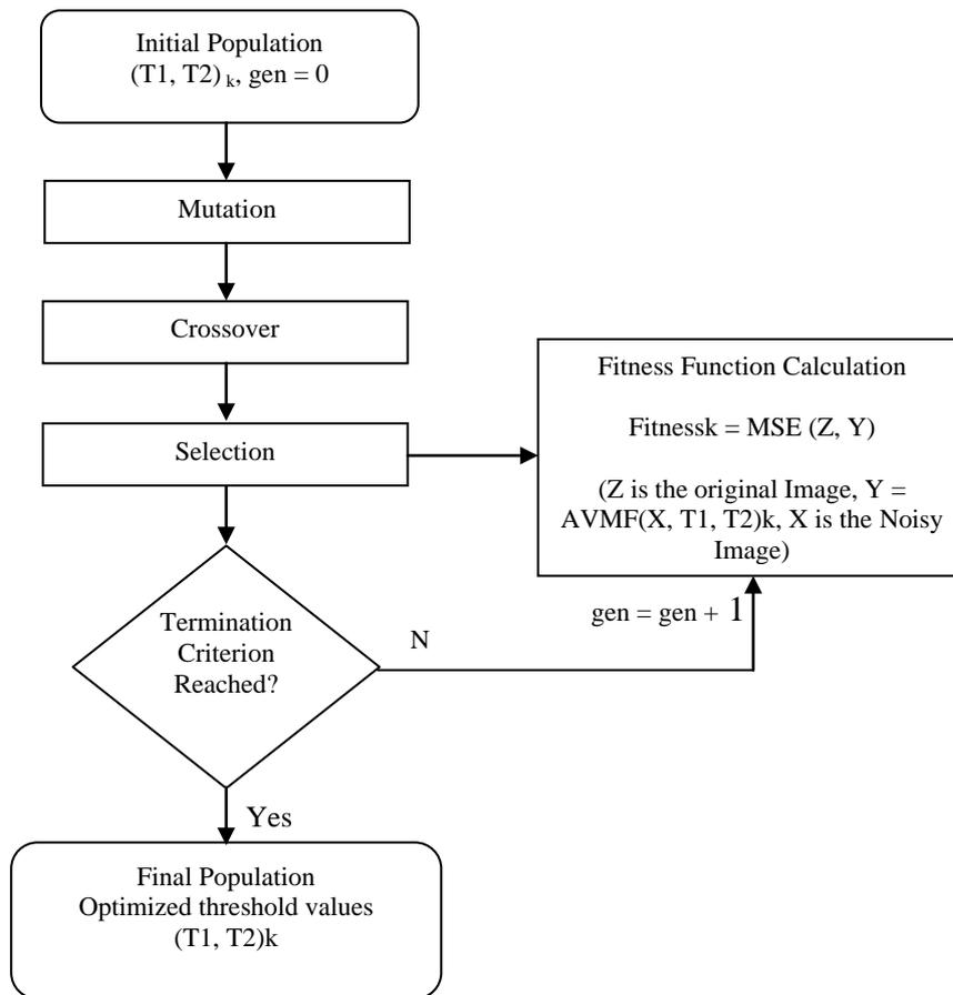
Fig 5. Optimized Threshold Value Estimation Procedure
