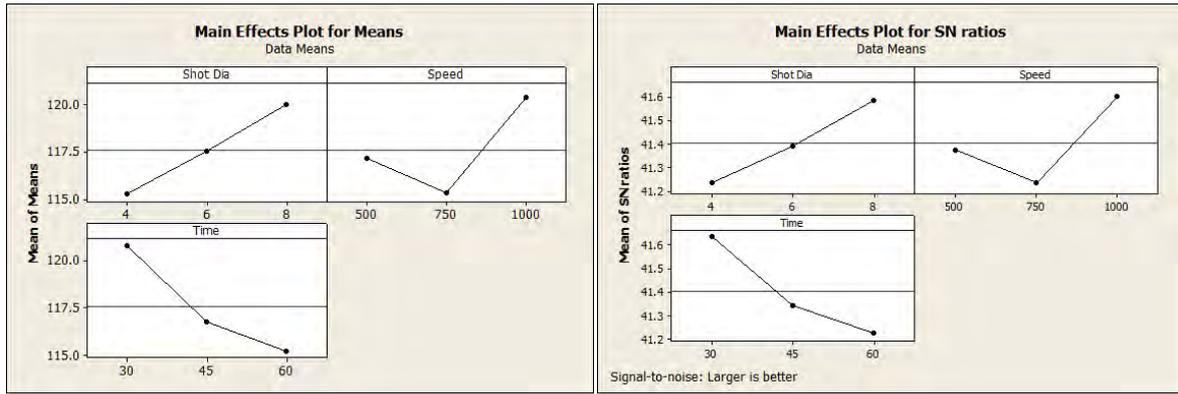
Fig. 2. Main Effects Plot for Means and S-N Ratios of Hardness
