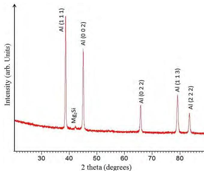
Fig. 5. XRD Pattern of AA6061 Treated by SSMT with the Process Combination of 8 mm Shots, 1000 Rpm Speed of Revolution and 30 Minutes Duration of Treatment
