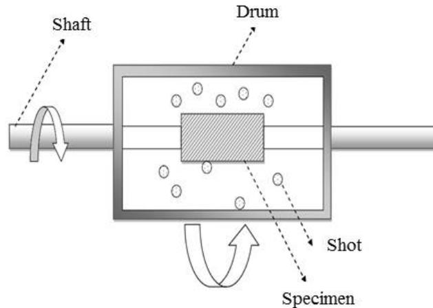
Fig. 1. Schematic Diagram of the Equipment Used for SSMT
