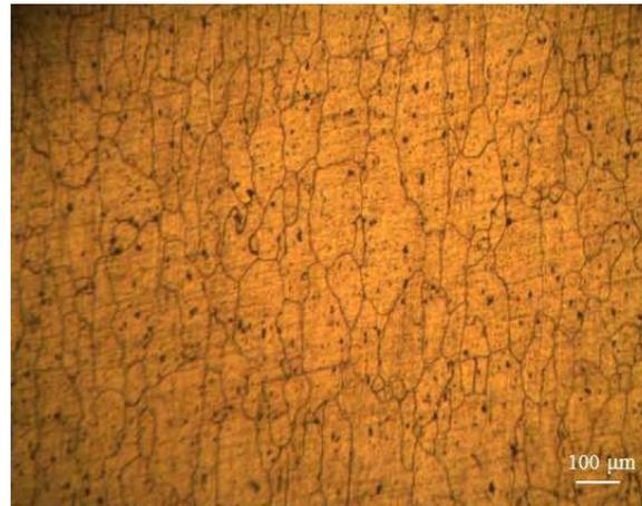
Fig. 4. Optical Microstructure of Untreated AA6061 (200x)
