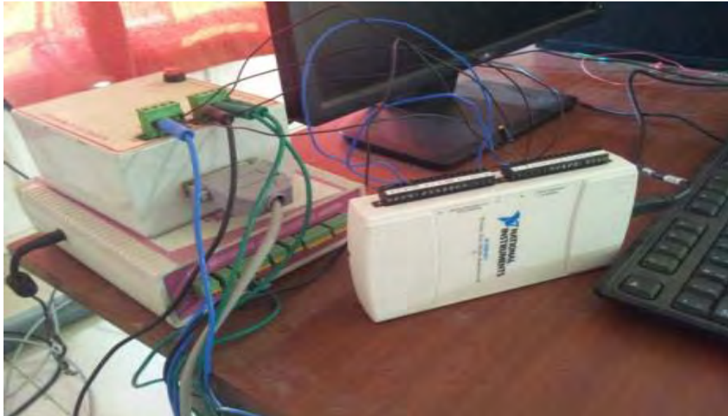
Fig.2. Interfaced NI-DAQmx 6211 data acquisition module card to the PC
