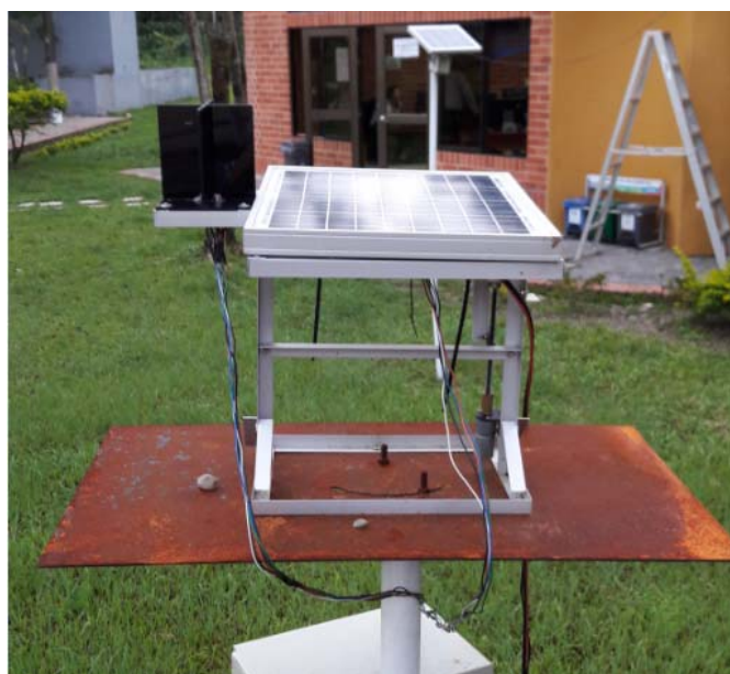
Fig. 4. One axis active solar tracking system
